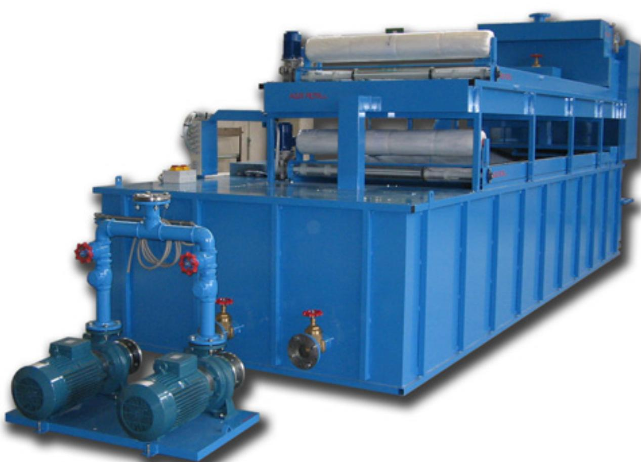
In our **C** type flat bed gravity strainers filtration occurs by **gravity** and the used filtering means is the **non woven fabric** capable to retain **contaminating particles of any kind, both metallic and non-metallic particles** produced by different industrial processes and found suspended in liquid lubrocoolants.
